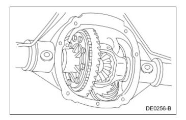
2. Install the originally removed differential bearing shim on the LH side.
