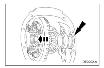
5. Using the Differential Shim Installer, fully seat the differential bearing shims.
